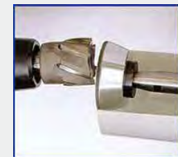
Grinding the clearance angles on the face
