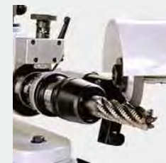
Grinding the flute rake angle
