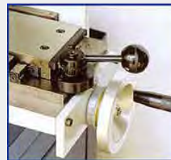
Rapid cross movement with hand lever.
