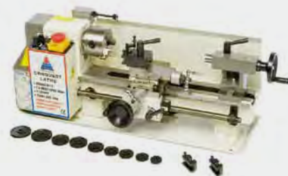
Conquest Lathe with Standard Thread Cutting Gears and Quick Change Toolpost Holders
