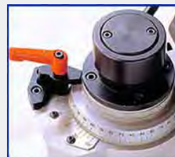
Fast and easy spiral set up variable from 0°~90° left or right hand
