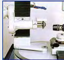
Rotary grinding head built into the machine base. Minimal travel required for the grinding process. Pivot point directly over the centre of rotary table. The grinding head can be easily set up for grinding the flutes, periphery, front rakes, cutting angles and relief angles.
