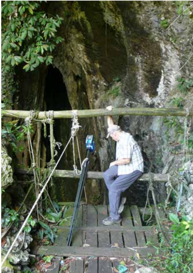
Challenging scans made possible by the Focus 3D X 330's ability to scan in oblique or horizontal positions.
