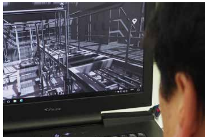
A technician working on a 3D model created with point cloud data that was obtained with the Focus 3D X 130.
